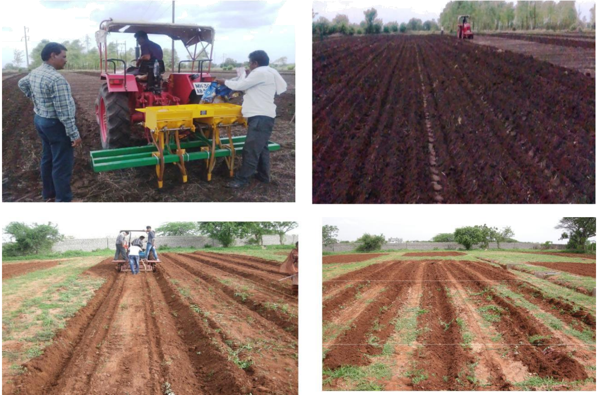
Fig: 2 Reshaping of a) Bed and furrow in Zero tillage b) Conservation furrow
